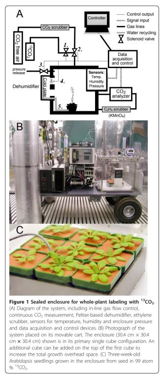
The design of the enclosure provided an environment where available  $CO_2$  had a high <sup>13</sup>C enrichment (~99%) for growing whole plants. This was accomplished by repeated purges of the complete system with  $CO_2$ -free air followed by a cycle of equilibration with 300 ppm <sup>13</sup>CO<sub>2</sub>, a second purge, and re-equilibration. This was
